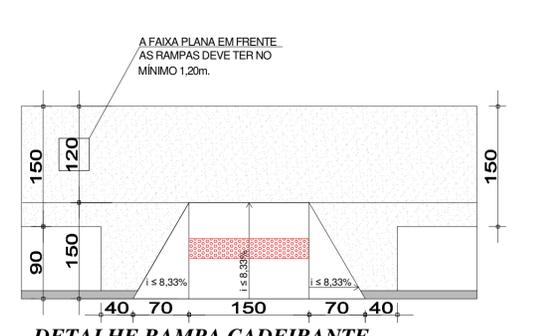
DETALHE RAMPA CADEIRANTE S/ ESCALA
