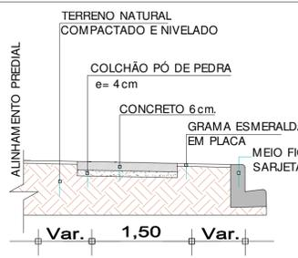
DETALHE TRANSVERSAL CALÇADA S/ ESCALA
